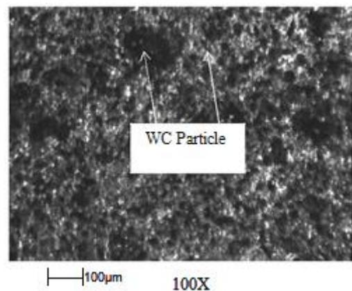
Fig. 19. Microstructure of WC and E-glass composite after machining by carbide insert.
