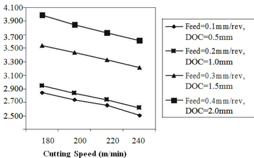
Fig. 5. Variation of surface roughness of WC and E-Glass composite using PCD insert
