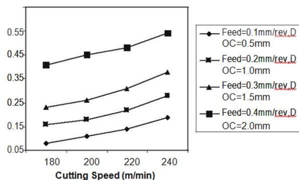
Fig. 11. Wear of carbide insert with cutting speed
