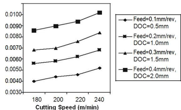
Fig. 13. Wear of PCD insert with cutting speed
