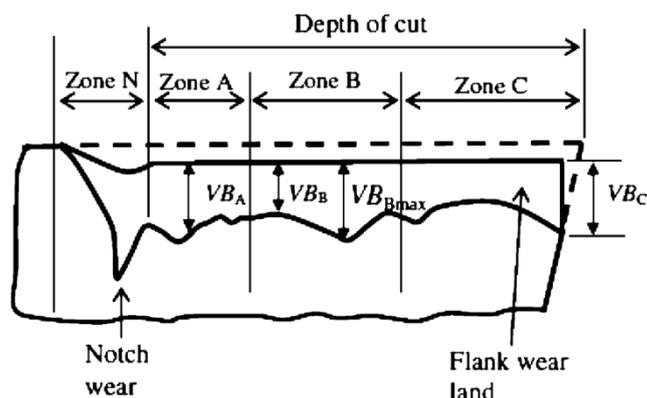
Fig. 10. Side view of cutting tool showing flank wear (ISO3685)
