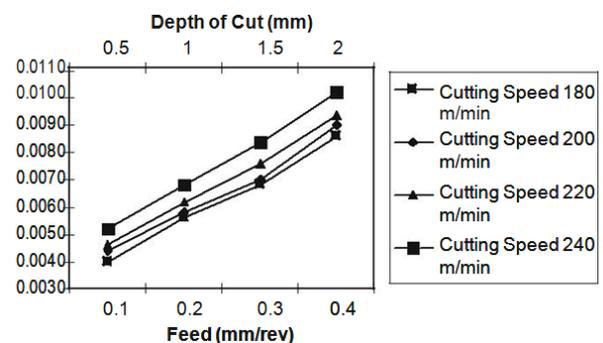
Fig.14. Wear of PCD insert with feed
