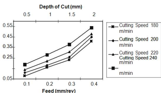
Fig. 12. Wear of carbide insert with feed
