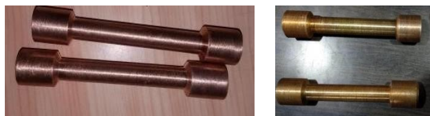
Fig 3: Specimens for tensile test
