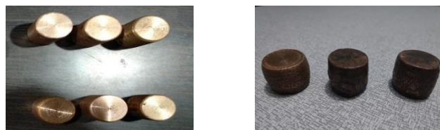
Fig 4: Specimens for compression test
