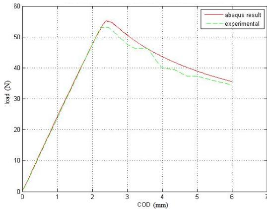
Fig 16: Load-deflection curve for multi directional DCB
