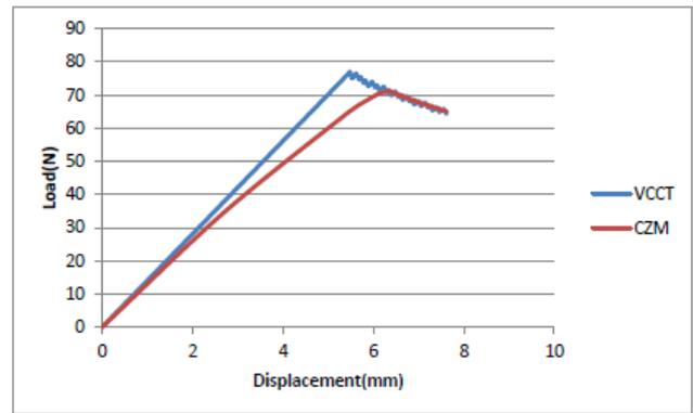
Fig 11: Load-displacement curves for VCCT and CZM
