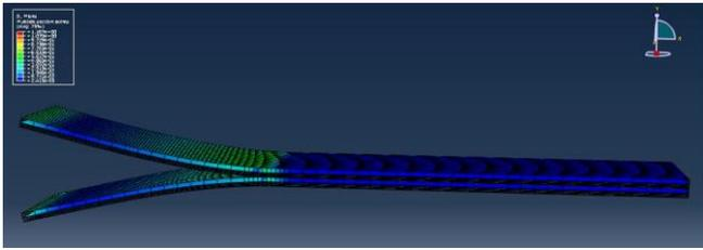
Fig 9: Crack Propagation of DCB specimen using VCCT technique
