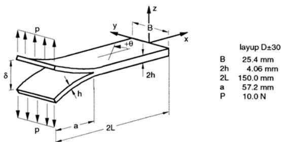
Fig 3 : Multidirectional Double Cantilever Beam specimen
