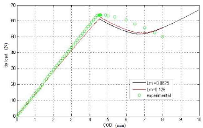
Fig 14: Load-deflection curve for the DCB specimen
