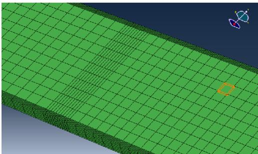
Fig 7 : Refine mesh at the crack tip
