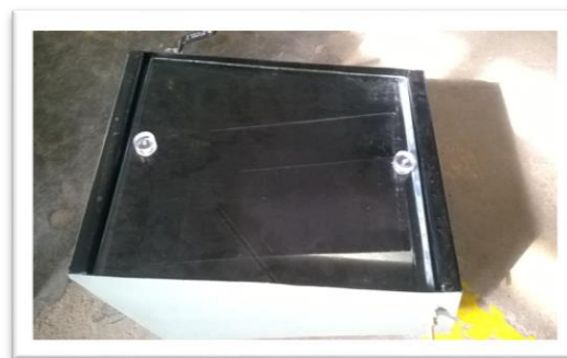
Fig.3 Top Cover with Glass
