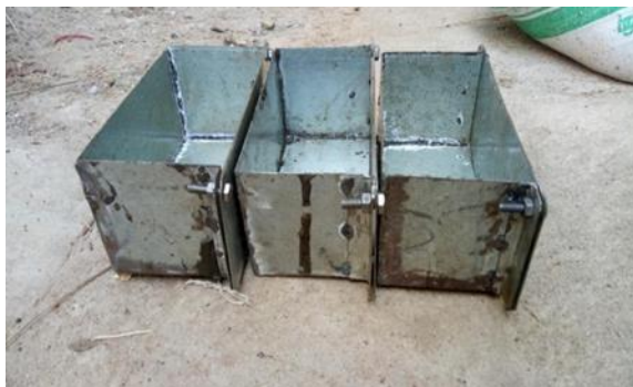
Fig 5. Mould of dimension (20 X 20 X 20) cm
