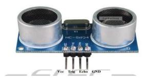
Ultrasonic device module consists of four pins:
