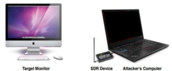
Figure 1: Hardware components of an EM eavesdropping attack on a computer monitor.
