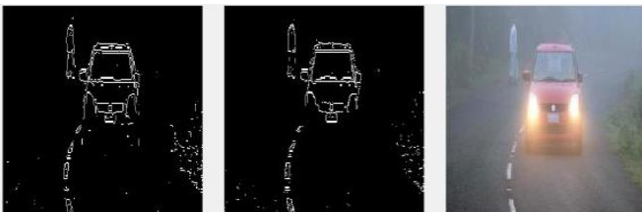
Figure 2. Original image to BW with edge detection.
