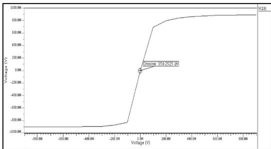
**Figure 11.** Offset Voltage of FDDTDC.
