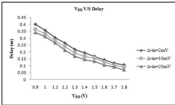
**Figure 17.** Delay v/s Supply Voltage.
