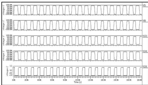
**Figure 10.** Transient Analysis of FDDTDC.
