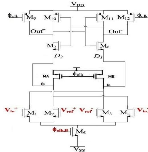
**Figure 2.** Fully Differential Double Tail Dynamic Comparator (FDDTDC).
