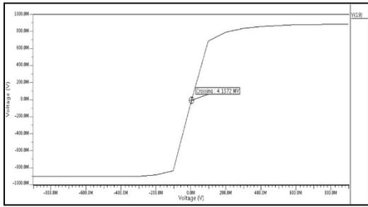
**Figure 5.** Offset Voltage of DDC.
