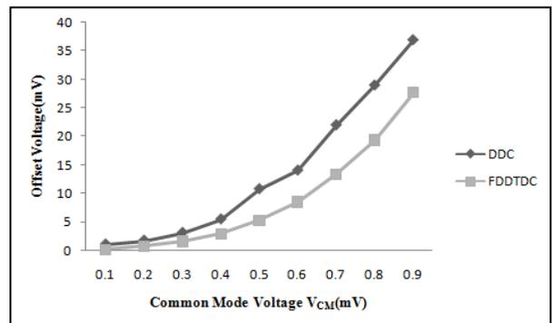
**Figure 16.** Common Mode Voltage v/s Offset Voltage.
