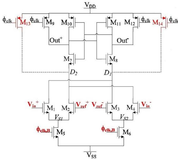
**Figure 1.** Differential Dynamic Comparator (DDC).[7]
