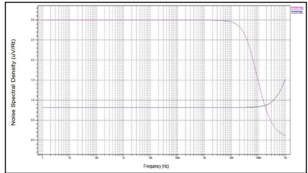
**Figure 13.** Input-Output Noise Spectral Density of FDDTDC
