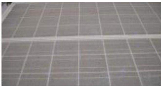
Fig 4 : Sun oriented module secured by substantial layer because of residue amassing before cleaning.
