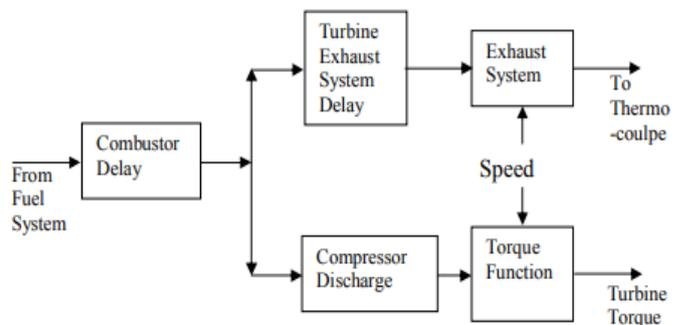
**Figure 8** Block diagram of compressor – turbine system
