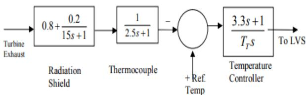
**Figure 6** Transfer function block diagram of temperature control loop
