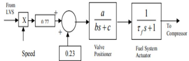
**Figure 7** Transfer function block diagram of fuel system
