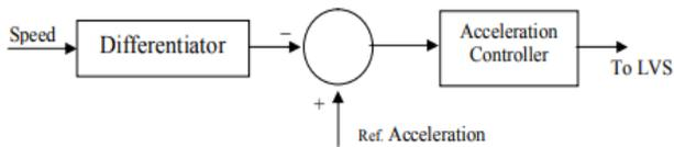
**Figure 5** Transfer function block diagram of acceleration control loop
