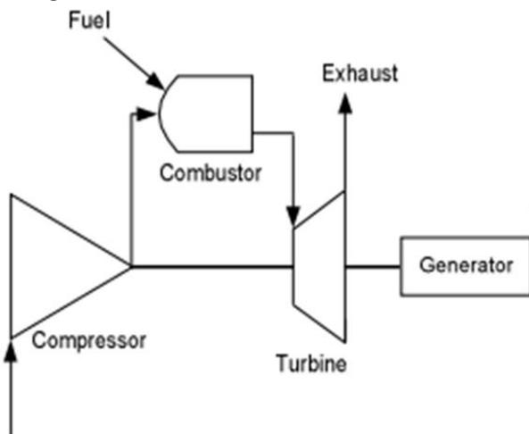
Figure 2 The schematic diagram for a simple cycle, single shaft gas turbine plant
