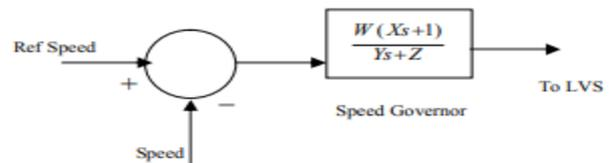
Figure 4 Transfer function block diagram of speed control loop
