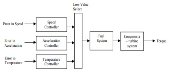
Figure 3. Block diagram representation of gas turbine plant
