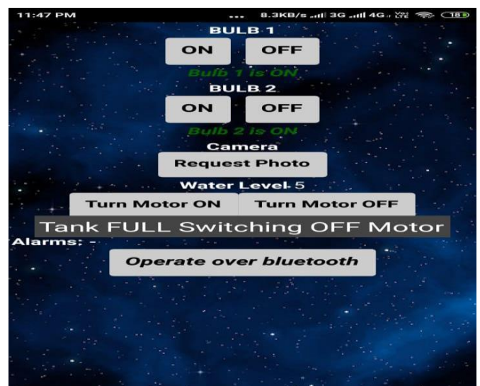
Figure 8 : Final Android App : Automatically Switching OFF the Motor.
