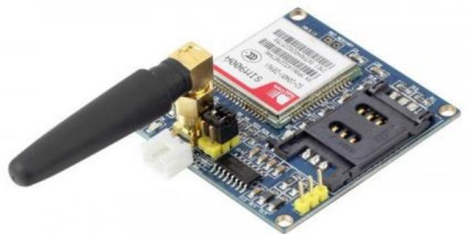
Figure 2. SIM 900a GPRS/GSM Module.
