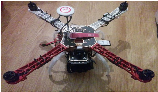
Fig.3.1.1. Quadcopter that is connected to the battery, camera, GPS tracker raspberry pi and other hardware parts.
