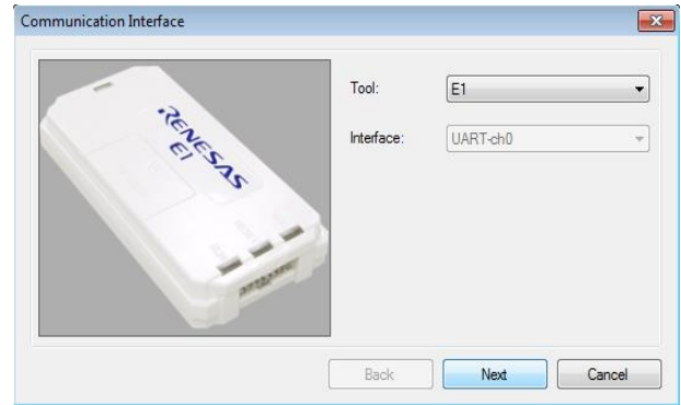
Figure 14: Flash programmer using Renesas flash programmer- choose emulator
