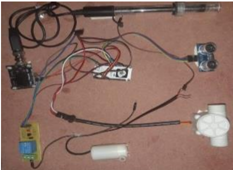
Sensors connection with Wi-Fi Controller
