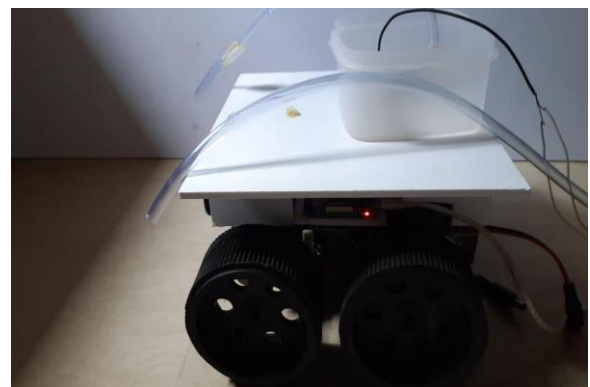
Figure 11: Robot with multiple extinguishing materials
