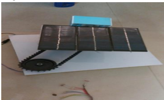
Figure.11: Connection of PMDC Motor to Solar Panel
