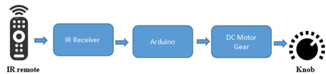
Fig. 2 Block Diagram of working of IR remote and IR receiver
