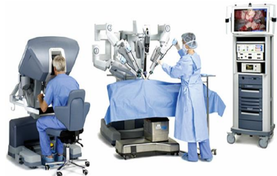
Fig 5. Components of Da Vinci System: Surgeons Console (left), Patients Cart (Centre), Vision Cart (Left) [22].
