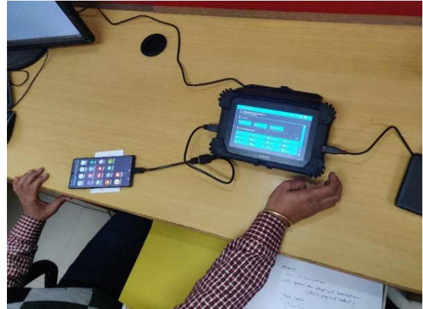
Fig. 6. Mobile Device analyzed using the UFED Touch-2-7.42
