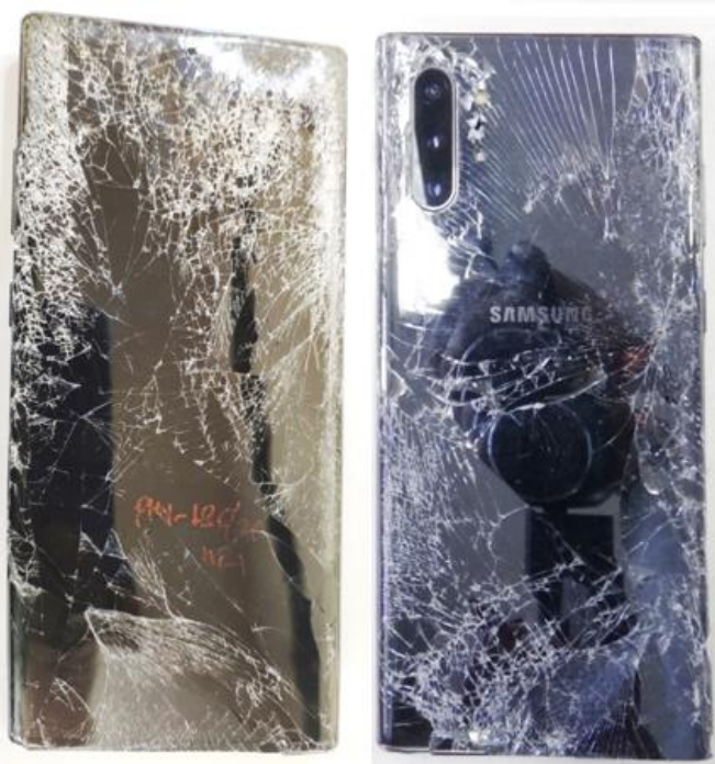
Fig. 1: Damaged Samsung Mobile Phone as delivered to the laboratory
