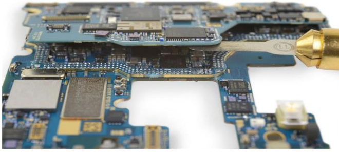
Fig.4: Silicon- Sandwich look of PCB Internally
