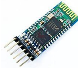
Figure 3. Bluetooth Module HS-06 [7]
