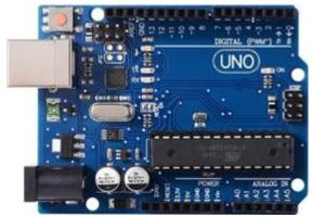
Arduino Uno is a microcontroller board based on the ATmeaga328P. it has 14 digital input/output pins, 6analog inputs, a 16 MHz ceramic resonator, a USB connection, a power jack, an ICSP header and a reset
