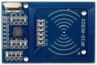
The RC 522 is a 13.56 megahertz RF ID module that is based on MFRC 522 Controller from NXP semiconductors full stop the model can support 12C, SPI and UART and normally H ship with are you for the card and key fob. It is commonly used in attendance systems and other person/object identification applications.
