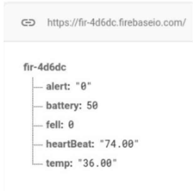
Figure 5. Logging the recorded values from vitals sensors on Firebase
