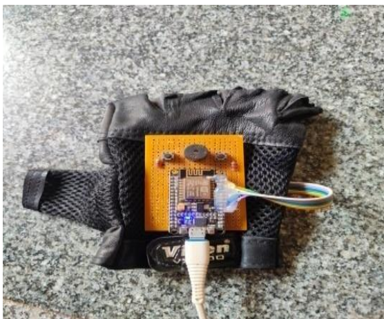
Figure 12: Buzzer on the RFID Hand Gloves
