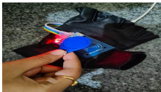
Figure 15: Tapping on RFID Tag
