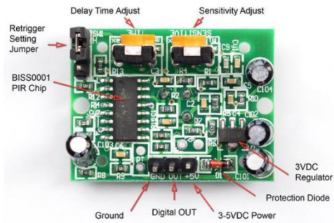
Figure 4: Passive Infra-Red Sensor and rear view
