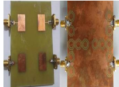
Figure-2 Fabricated Type-I MIMO Antenna
