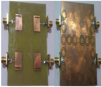
Figure-5 Fabricated Type-II MIMO Antenna
