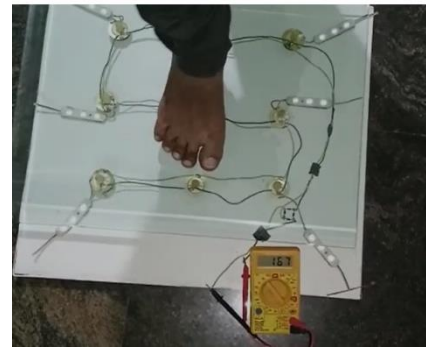
FIGURE 7: LEDS GLOWING WHEN PRESSURE IS APPLIED
