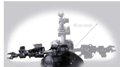
FIGURE 4.3 A PIONEER ARM REDUNDANT MANIPULATOR
