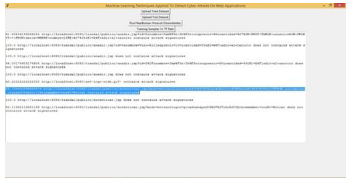
Fig 4.4 In above screen in selected text u can see first contains similarity score between train request data and test request data and then request data is displaying and then showing whether its normal or contains attack signatures.
