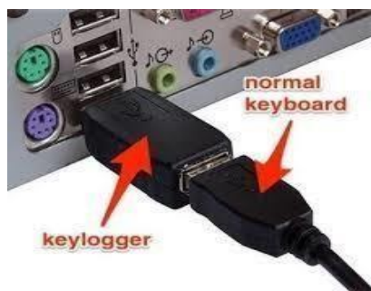
Figure 3 Representation of Hardware Based Keylogger They don't depend upon any software being installed as they function at hardware level in a computer system. The hardware Keyloggers cannot be detected
