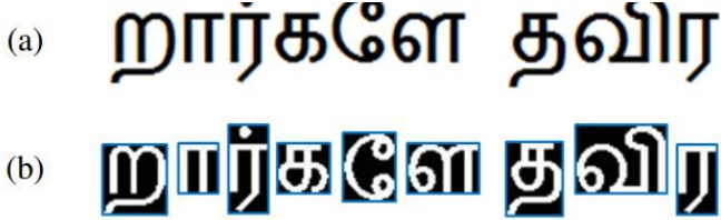
Figure 12: Segmentation of Tamil characters (a) Original image (b) Segmented characters
