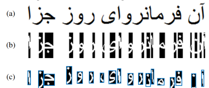
Figure 4: Segmentation of Arabic characters from Arabic text line (Thabit Font) (a) Original text image (b) Edge identification (c) Segmented characters
