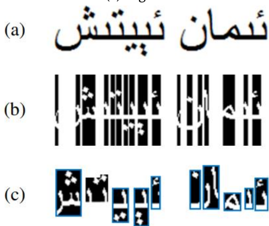
Figure 7: Segmentation of Uyghur characters (a) Original image (b) Edge identification (c) Segmented characters
