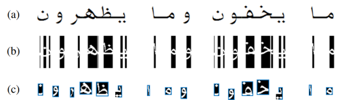
Figure 4: Segmentation of Arabic characters from Arabic text line (Thabit Font) (a) Original text image (b) Edge identification (c) Segmented characters
