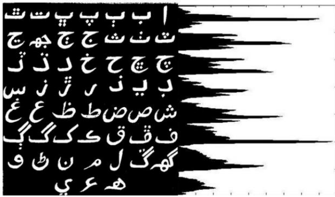
Figure 2: Projection Method used in Sindhi (Hakro, 2015)
