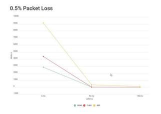
Our research project embarked on an in- depth analysis and testing of the BBR congestion control algorithm, comparing its performance against traditional algorithms such as Reno and Cubic, particularly under conditions of high packet loss. The findings from our tests have provided valuable insights into the capabilities and advantages of BBR in challenging network environments.
