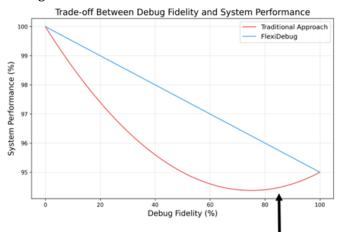
This line plot illustrates the trade-off between debug fidelity and system performance in 5G networks. It compares the traditional approach with the FlexiDebug framework proposed by Kumar et al. (2023), showing how FlexiDebug achieves a better balance between debugging capability and system performance.
