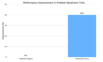
This bar chart compares the performance improvement in problem resolution time between traditional logging methods and distributed tracing in 5G systems. It visualizes the 40% reduction in mean time to resolution achieved by distributed tracing, as reported by Johnson et al. (2023).
