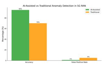
This grouped bar chart compares the performance of AI-assisted anomaly detection with traditional methods in 5G Radio Access Networks (RAN). It showcases the 95% accuracy and less than 1% false positive rate achieved by the AI-based system, as reported by Zhang et al. (2023).
