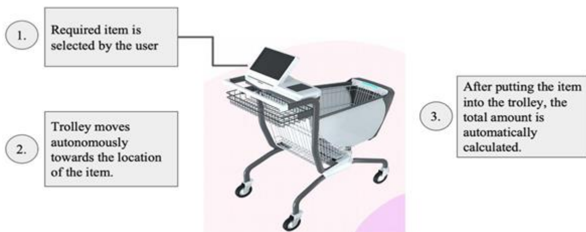
FIGURE 1. The overall design of our model is represented in the block diagram
