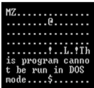
Figure 3. (Shows 'MZ' is the first two letters) Figure 4. (Shows PE header of suchost..exe)
