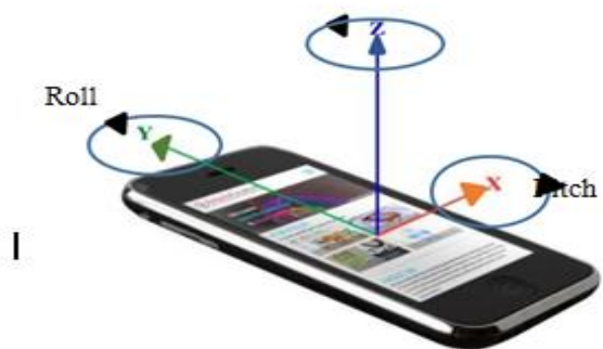
Fig 3. Gyroscope Axes on Smartphone
