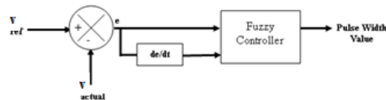
Figure 3. Schematic diagram of fuzzy controller
