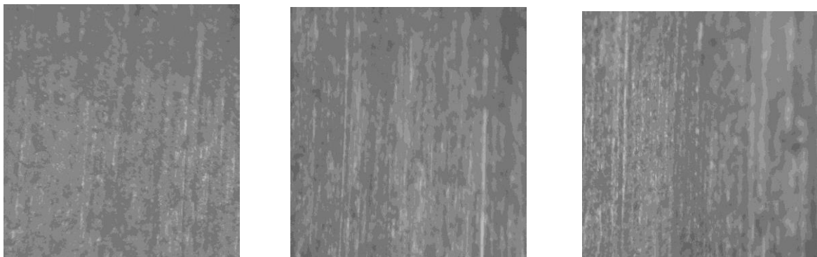
Figure 4: Microstructures of the test specimens run for 246m sliding distance and 3 N applied load The microstructure is typical of Aluminum alloy with small particles of Silicon and Magnesium in Aluminum solid solution.
