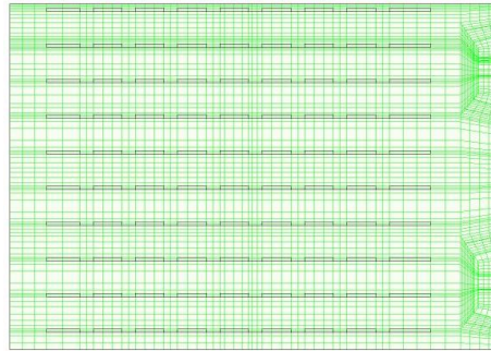
Fig.2: Cut plane of Hexagonal meshed model
