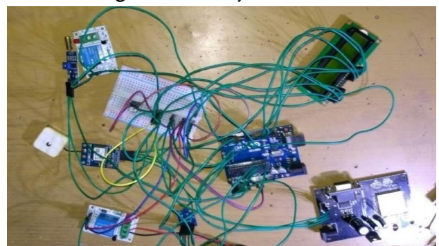
Figure 3. Interfacing of GSM and GPS with Arduino
