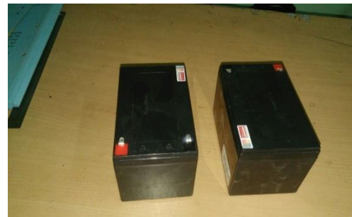
Figure 7. Lead acid battery
