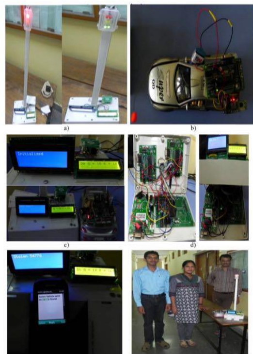
Figure 5. Proposed model images transmitter and receiver. (a) Pole status at different condition. (b) Transmitter (ZigBee). (c) LCD display at receiver. (d) Detailed image of receiver. (e) When stolen vehicle is detected. (f) Working model.
