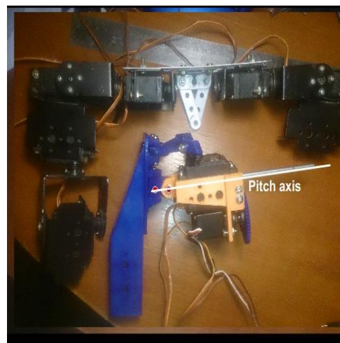
Figure 5. Pitch axis rotation
