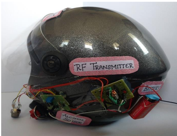
Figure 1. Helmet Unit Affixed With Alcohol Sensor, Touch Sensor and RF Transmitter
