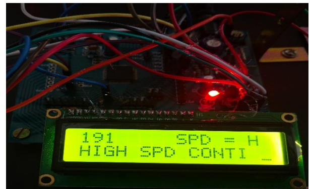
Figure 4. When rider exceeds the speed limit, the alert message “High Speed Continued” is displayed
