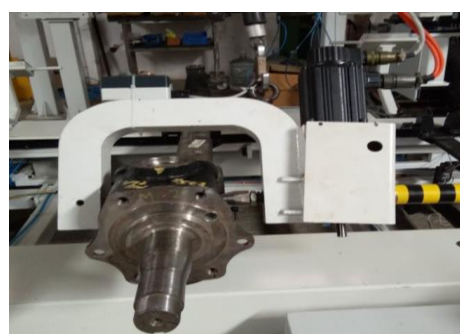
Figure 1.3 cotter pin insertion [rear view]
