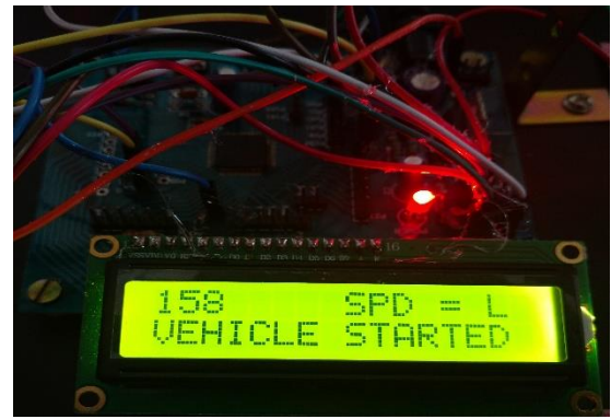
Figure 3. When Helmet Is Worn and No Alcohol Content Is Detected, the Vehicle Unit Starts
