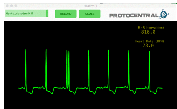
Figure 6. ECG signal acquired through conductive fabric.
