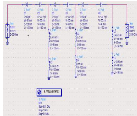
Figure 3 Lumped element High pass filter (N=3)
