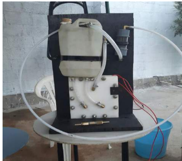
Fig.8. Oxy-hydrogen generator system
