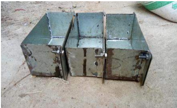
Fig 5. Mould of dimension (20 X 20 X 20) cm
