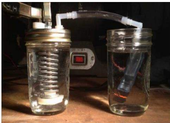
Fig.1 Wet cell generator
