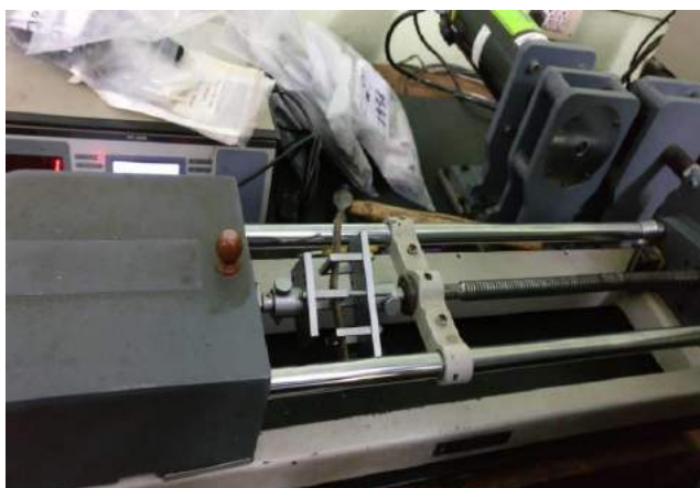
Fig 5. Tensile testing of the specimen
