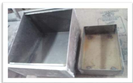
Fig. 1 Outer and inner tank made by bending and arc welding
