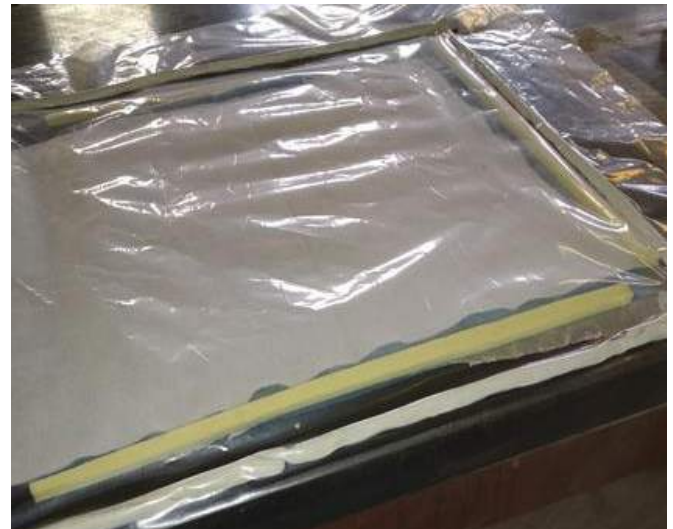
Fig 3. Vacuum bagging process
