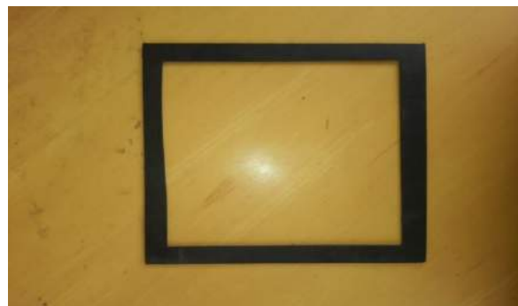
Fig. 4. Neoprene Gasket cut in shape
