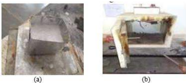
Figure 4. (a) Pouring colloid into sheet metal model (b) Sheet metal model is placed in oven
