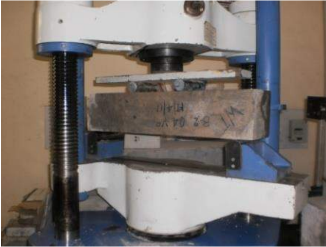
Split tensile test
