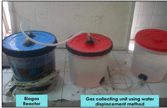
Fig. 1. Pictorial view of biogas reactor
