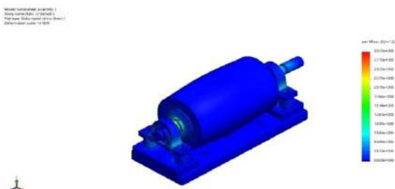
Fig. 8: Chamfering wheel assembly 1-Static 2-Stress-Stress1
