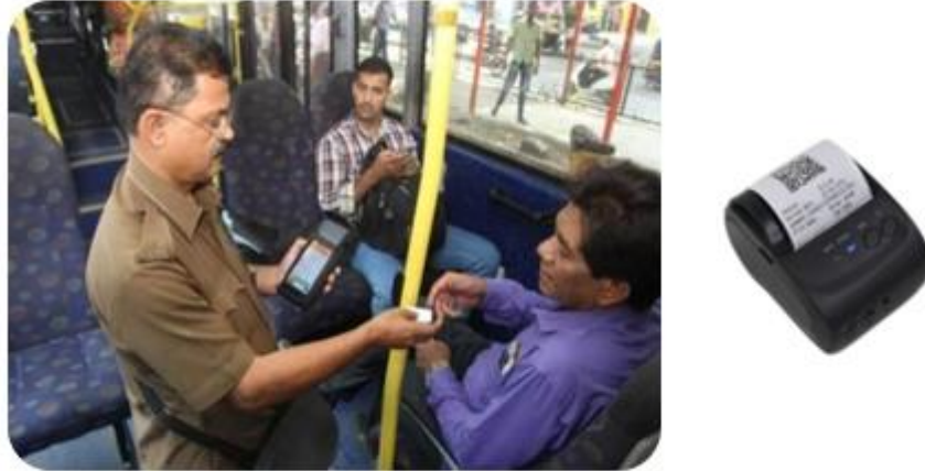
Figure 19. Conductors can use the conductor app to generate and print ticket for users who don't have access to smartphones, using handy Bluetooth printers.
